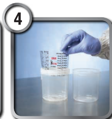
If not using a scale to measure, insert 3M™ PPS™ mix ratio film into cup before inserting liner in order to measure the paint according to paint manufacturer's guidelines.
