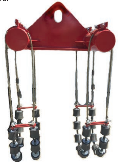
24 Inch Four Strand Cradle PN 2004 12-24 inch pipe capacity 28,000 lbs capacity 28 rollers per cradle
