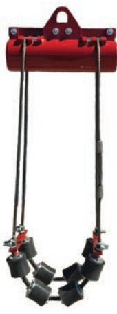
12 Inch Double Strand Cradle PN 2002 6-12 inch capacity 17,000 lbs capacity 8 rollers per cradle
