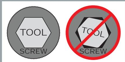
Every Bondhus tool is designed and machined to achieve an optimal fit between tool and fastener. Tools insert quickly and easily into screw head and fit snug to generate greater torque and minimize slippage and stripping.
