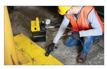
This PED-1101B Submerged pump quickly and quietly powers Enerpac's hydraulic Nut Cutter in this maintenance application.
