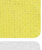
However, because it is an open-weave knit material, Kevlar® is susceptible to small punctures through the knit penetrating the skin. This has resulted in severe injury with punctures through a glove, tearing the skin. Ultraviolet exposure and temperature extremes also degrade the fibers, resulting in declining performance over time.
