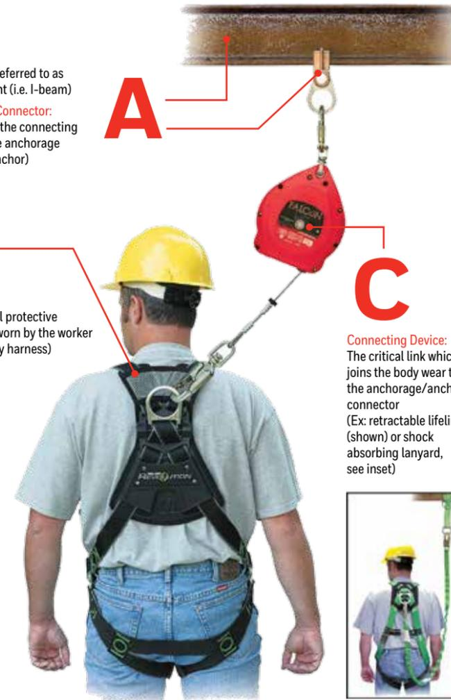
**3 key components of the Personal Fall Arrest System (PFAS) must be in place and properly used to provide maximum worker protection.**
