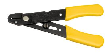
Klein Tools' 1003 Wire Stripper and Cutter is a handly, light, compact tool for stripping 12-26 AWG solid and 14-28 AWG stranded wire. Features convenient hole for looping or bending wire. Adjustable slide stop with set screw for repeat stripping work.
