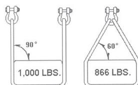
Sling capacity decreases as the angle decreases. A sling capable of lifting 1,000-lbs. in a 90° vertical basket hitch can only lift 866-lbs. at a 60° angle.
