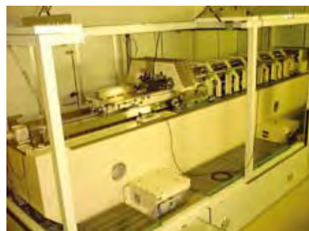
Ultra-precision length measuring machine with vacuum laser interferometer
