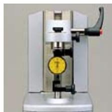
Using test indicator attachment set (02ASK000)
