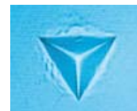
Indentation by triangular pyramid indenter
