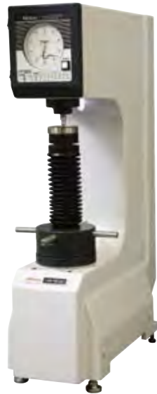
HR-210MR 963-220 Rockwell hardness testing machine Manual weight changing (with total test force selected) and handling of preliminary test force. Motor drive controls loading sequence.
