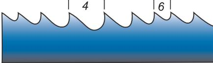
For most metal sawing applications. Multi pitch blades vary tooth spacing between two extremes.
