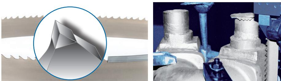
Set tooth tungsten carbide for cutting highly abrasive materials.
