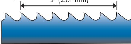
For fast cutting materials. Single pitch blades have consistent tooth spacing. The number of teeth per one-inch length is the TPI.
