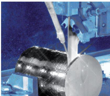
For sawing extremely brittle and abrasive materials.
