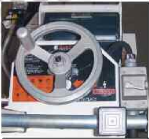
CC1500 Operator view showing the heavy duty screw feed raise/lower
