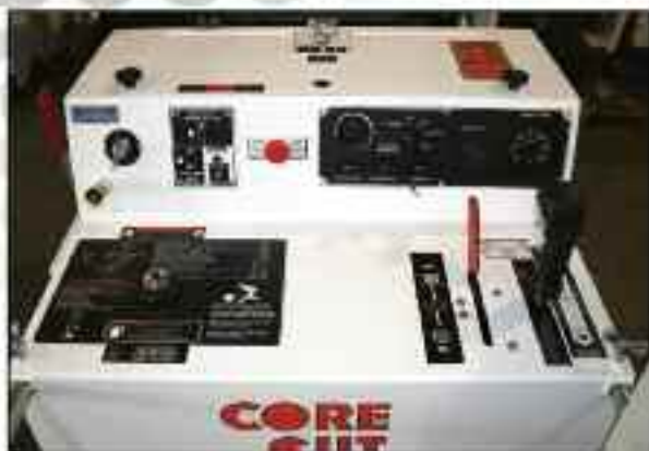
Mini-Groover control panel with power raise and lower controls, drive control and gauges
