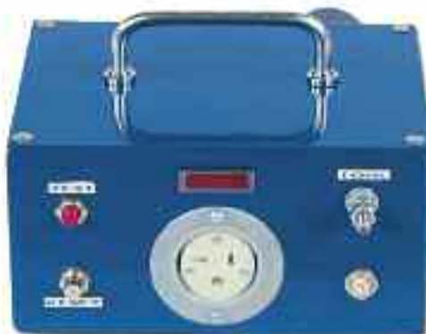
Core Bore Stop Box Shuts off the electricity to the motor(s) if the core bit hits grounded metal
