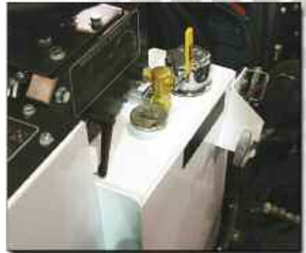
Upgraded, larger hydraulic oil tank
